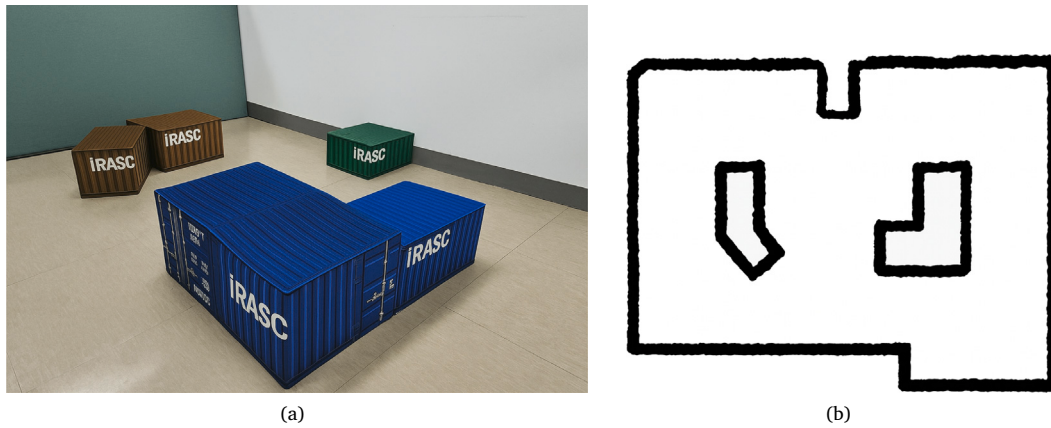
Fig. 8. Comparison between (a) the real experimental environment and (b) the SLAM-generated map.
